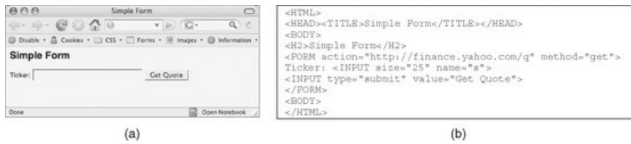
Figure 3.3 A web form (a) displayed in a browser and (b) the HTML that creates the form.
